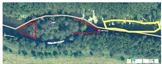
Figure 4.9 Proposed solution for moving the sediments in the riverbed to the existing the islet in the riverbed
