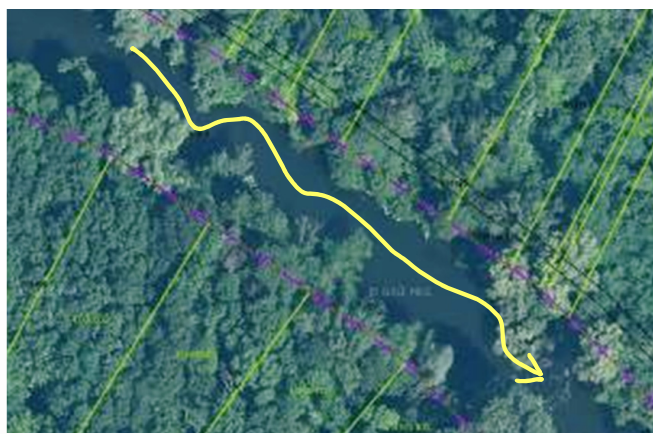
Figure 4.13 Changing the flow regime in the stream by creating sediments on riverbanks around fallen trees
