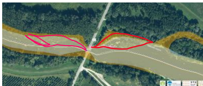
Figure 4.1 Proposal for the placement of gravel benches
