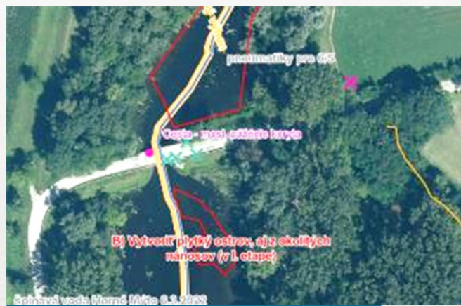
Figure 4.11 Proposed solution for moving sediments in the riverbed and creating gravel benches
