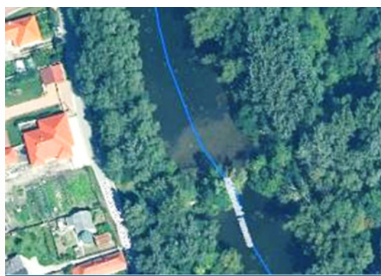
Figure 4.18 A flow blockage formed by the ruins of an old road bridge on the stream
