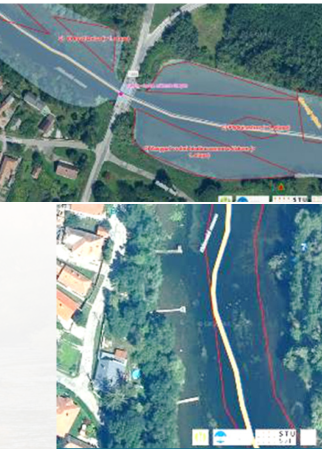
Figure 4.7 Proposed solution for moving sediments in the riverbed and creating gravel benches
