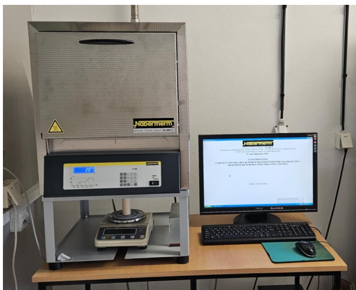
Obr. 2 Gravimetrická pec Nabertherm L9/11/SW/P330 s príslušenstvom Fig. 2 Gravimetric furnace Nabertherm L9/11/SW/P330 with accessories
