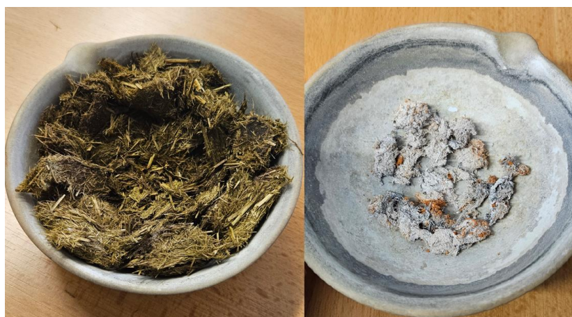
Obr. 5 Vzorka biopaliva kanského trusu pred experimentom a po experimente Fig. 5 Sample of horse dung biofuel before and after the experiment
