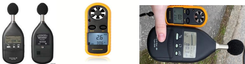
Obr. 3 Meracie prístroje: a) hlukomer, b) anemometer, c) prístroje počas meraní Fig. 3 Measurement devices: a) noise meter, b) anemometer, c) devices during the measurements
