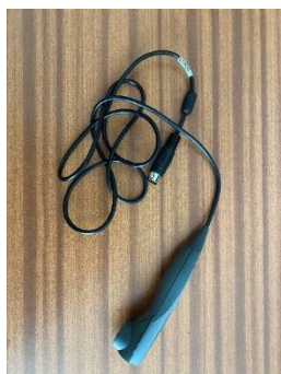
Obr. 2 Sonda na meranie CO Fig. 2 Measuring probe CO
