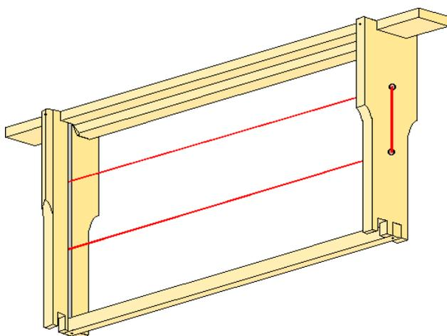
Figure 25 Wooden wired bee frame
