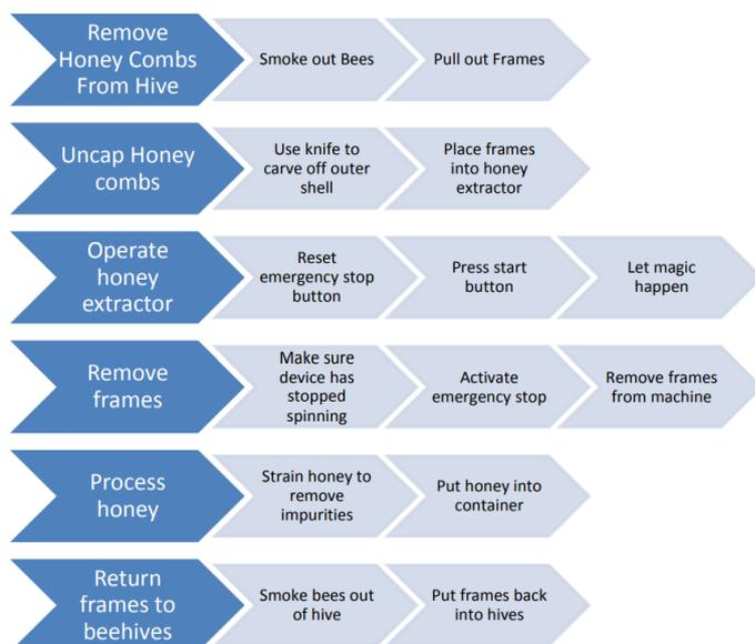
Figure 83 Flow chart for operation of honey extractor
