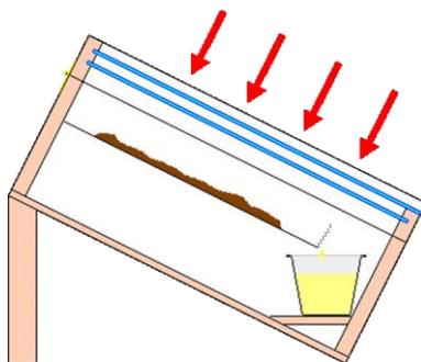
Figure 89 Solar wax melter
