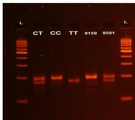
Fig. 1 Illustration of MTHFR rs1801133 genotypes on agarose gels
