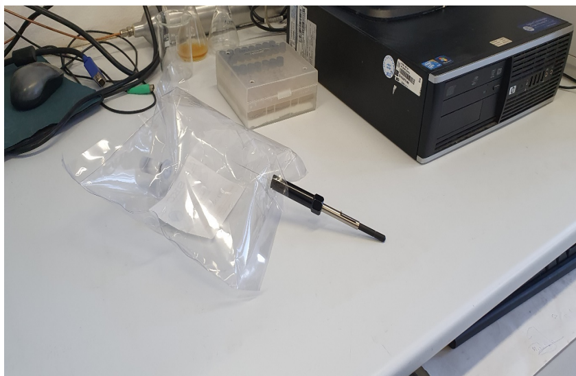
Figure 6.1 Extraction of volatile compounds to SPME fiber from air sampled to plastic box
