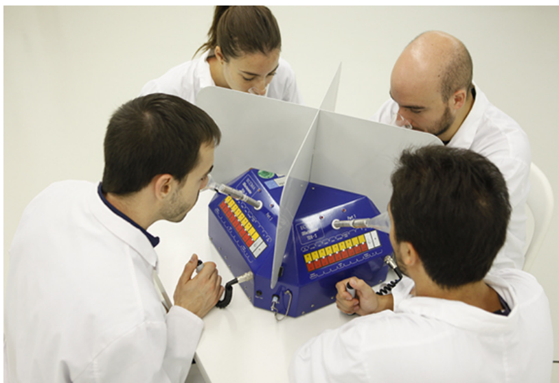
Figure 4.2 Olfactometry in laboratory conditions
