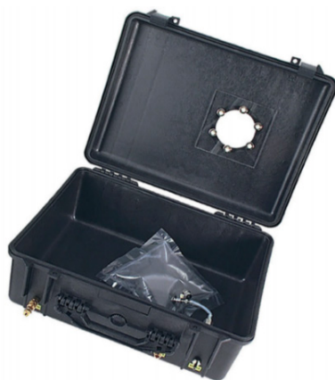
Figure 1.6 Special suitcase for sampling air bags
