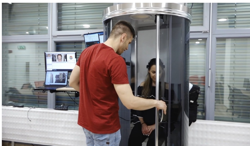
Figure 4.8 Special aromatization box for aroma testing
