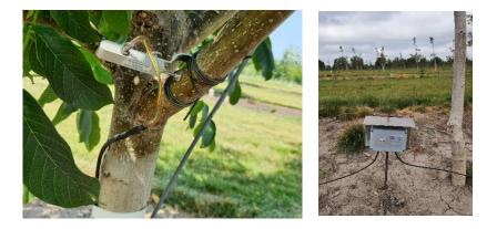
Figure 3 Diameter dendrometer small and datalogger DL-18 (source: Kováčová, 2020)
