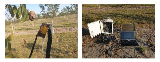
Figure 2 Sap flow measurement equipment (source: Kováčová, 2019)
