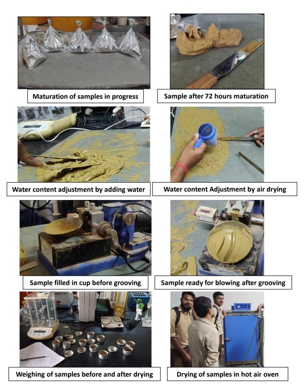
Figure 3 Pictorial representation of various stages of liquid limit test
