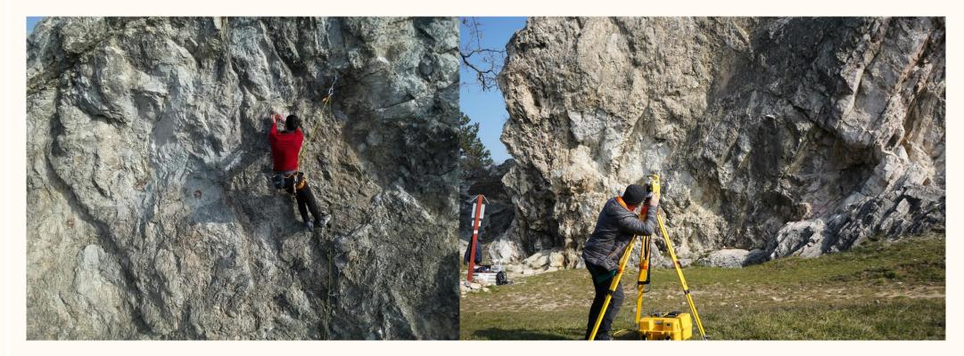
Figure 2. Installing and measuring the control points
