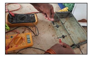
Figure 6 Measurement of tap water resistivity
