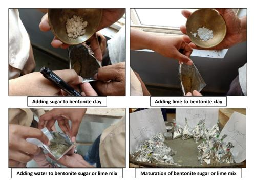
Figure 2 Pictorial representation of various stages of sample preparation
