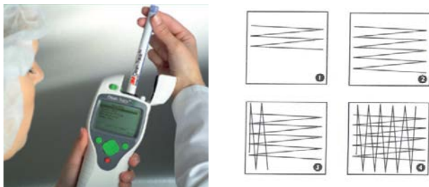
Figure 1 The HY-LITE NG system from Biotrace and procedure for taking surface ATP sample
