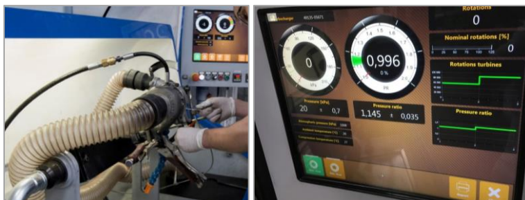
Obr. 7 Meranie tlaku turba a nastavenie variabilnej geometrie Fig. 7 Measuring turbo pressure and setting variable geometry
