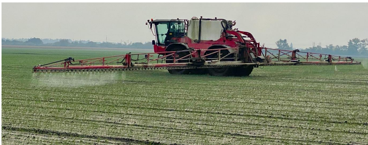
Obr. 2 Postrekovače Agrifac Condor CO4 pri variabilnej aplikácii (Foto autor) Fig. 2 Sprayer Agrifac Condor CO4 during variable rate application (Photo author)
