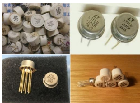
Obr. 1 Integrované referenčné obvody LM399, LTFLU, LTZ1000, MAB399 Fig. 1 Integrated reference circuits LM399, LTFLU, LTZ1000, MAB399
