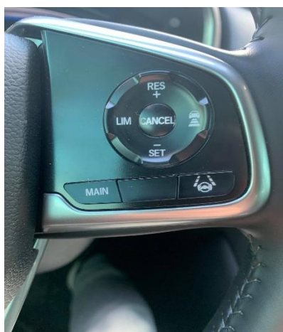
Obr. 7 Nastavenie line asistenta na volante Hondy CR-V Fig. 7 Setting of line assist on steering wheel on Honda CR-V
